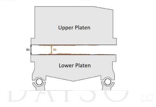
Unevenness because of rust and dirt also occurs on the plates of the upper chase and the lower counter die-cutting bed (Fig. 2 - 5).
