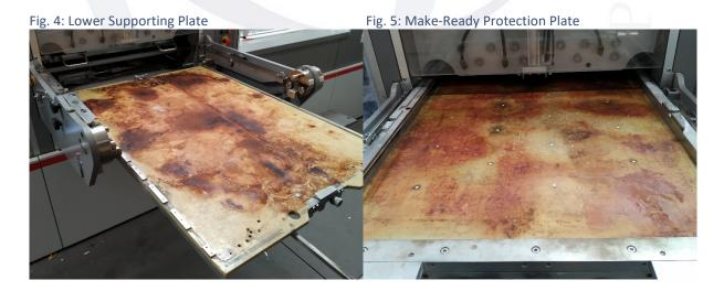
Residues of patch-up tape or adhesive tape for fixing the make-ready sheet also means unevenness on the chase and make-ready protection plate (Fig. 6). These in turn become effective during die-cutting.
