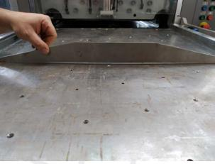
hair & dust development as well as burst folds ( $\rightarrow$  no centering between creasing rule and creasing matrix). In addition, bent cutting plates lead to increased set-up times in order to reach the register.
