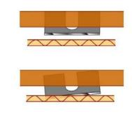
The cutting and creasing rules are subject to the general manufacturing tolerances and cannot be influenced. For example, the height tolerance for rules is e.g. approx. +-0.02mm. Therefore, these tolerances must continuously be patched up.
